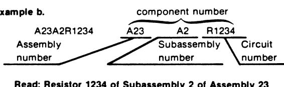
Only the circuit number will appear on the diagrams and circuit board illustrations. Each diagram and circuit board illustration is clearly marked with the assembly number. Assembly numbers are also marked on the mechanical exploded views located in the Mechanical Parts List. The component number is obtained by adding the assembly number prefix to the circuit number.
